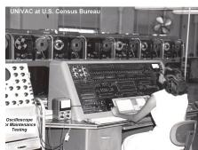
UNIVAC used 5,000 vacuum tubes, weighed 8 tons, occupied 380 square feet, used 125kW of electricity (your home uses, on average, 1.2kW), and could perform 2000 operations per second. (Such as adding 1 + 1 = 2).
